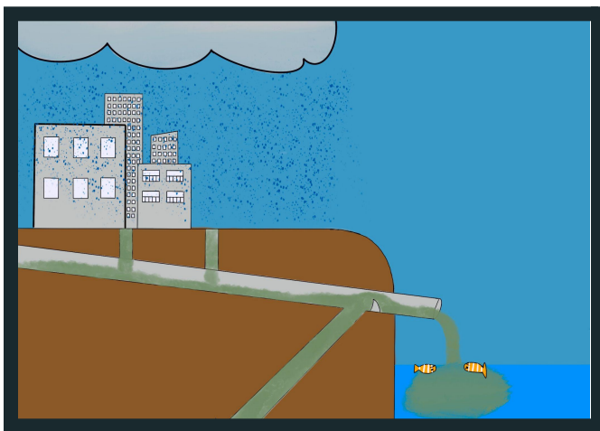
Figure 1: Alvarez, K. (2023) CSO leaking into local river
